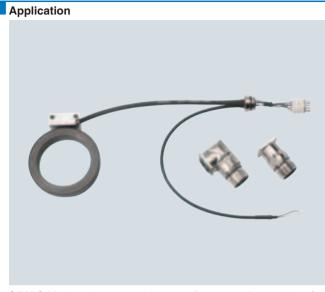
SIMAG H2 is an incremental system for measuring angles of rotation and rotational speeds. The application range comprises hollow-shaft applications with direct drives, as well as autonomous spindle encoder applications.
