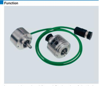
Incremental encoders deliver a defined number of electrical pulses per rotation, which represent the measurement of the traveled distance or angle.
