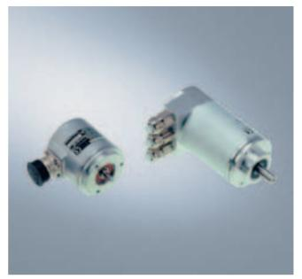
Absolute encoders (absolute shaft encoders) are designed on the same scanning principle as incremental encoders, but have a greater number of tracks. For example, if there are 13 tracks, then  $2^{13} = 8192$  steps are coded in the case of single-turn encoders. The code used is a one-step code (gray code), which prevents any scanning errors from occurring.
