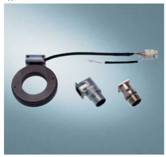
SIMAG H2 is an incremental system for measuring angles of rotation and rotational speeds. Applications include hollow-shaft applications with direct drives 1FE1 and 1PH2 as well as applications as an autonomous spindle encoder. SIMAG H2 is intended to replace the SIZAG 2 hollow-shaft measuring system in new applications.
